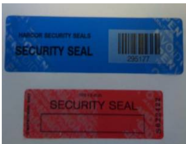
Image 2: Security Seals following attempts to remove them
